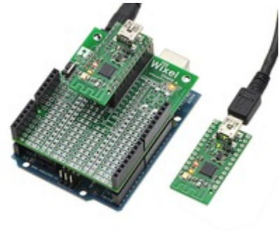
Wixel shield for Arduino powered through its power jack, communicating wirelessly with another Wixel.
