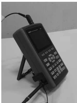
Picture 3-2 Compensation Signal Output Connection of the Apparatus
