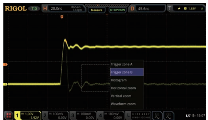
Draw a rectangle on the transient exception signal and select Trigger zone A.
